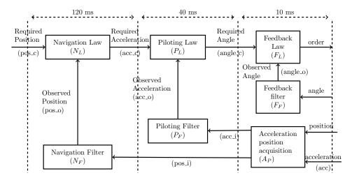
Figure 2: Flight control system
