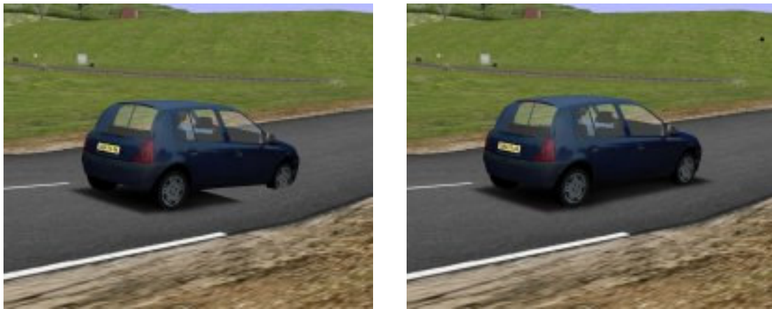
Figure 3: Example of graphical glitches corrections brought by RND in SCANeR ® II
