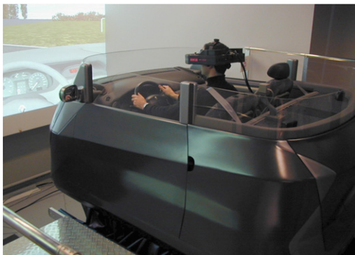
Fig. 5. Left, one of Renault's driving simulators: the user, wearing a virtual reality helmet, drives in the simulation using a real car's cockpit. Right, a screenshot of SCANER TM , the application used at Renault, where the scenario involves confronting the driver to a risky situation while driving on snow, with limited car adherence.
